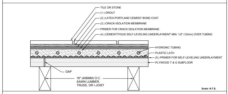
Drawings are developed to be compatible with Tile Council of North America 2013 TCNA Handbook for Ceramic, Glass and Stone Tile Installation.
