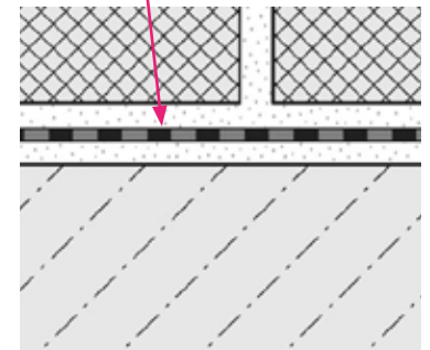
ARDEX TLT™ Waterproofing Membrane = 5 mil thick
