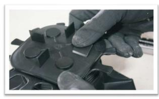
Cut the bottom of the pedestal with a hand grinder or similar tool.
